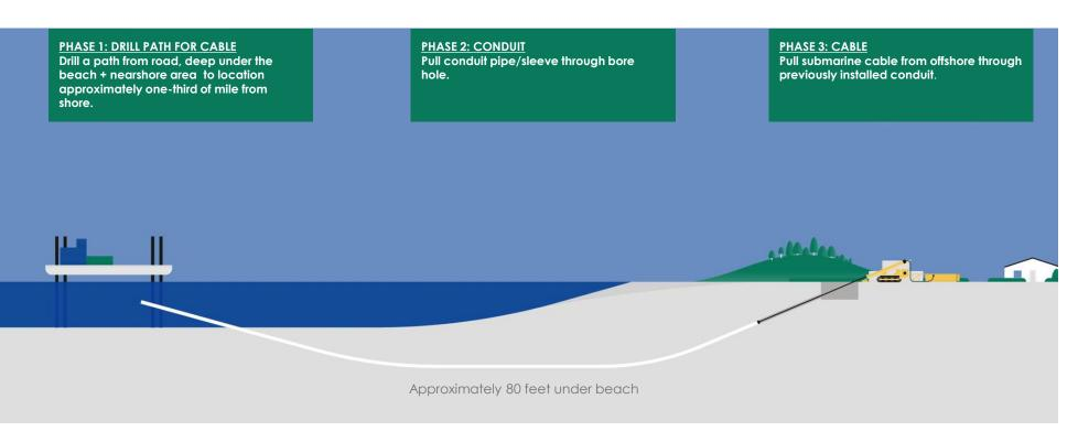
This an overview of the Horizontal Directional Drilling Process (HDD) that will be used to set the wind farm's power cable deep beneath the beach and nearshore area.
