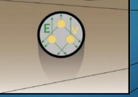
Magnetic field (B) surrounds electric current (I) on conductors and is not appreciably blocked by the metal sheath. The oscillating magnetic field induces a weak electric field (E) outside the cable.
